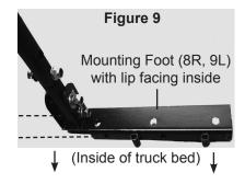
14. Please note: If lower Truck Rack height is desired, Leg Stands can be fastened directly to Front and Rear Mounting Feet without Coupler Risers. Use Bolts (27), Nuts (28), Spring Washers (29) and Flat Washers (30) to fasten Leg Stand to Feet. See Figure 10, below.
